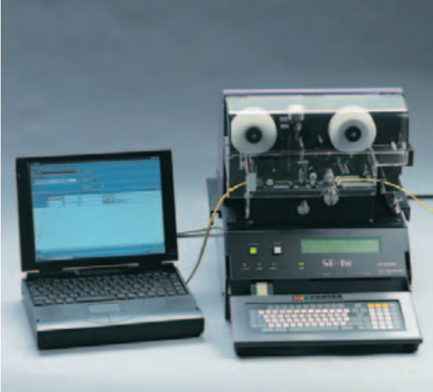
SP1W Marking machine for high volume on site marking production. For further information.
