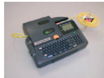
PRINTING ON PROFILE FROM A COMPACT DISC, MOUNTED ON THE REEL BRACKET.
